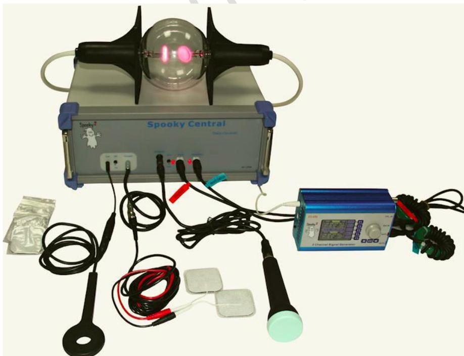
1.1.1. Connect your generator to Spooky Central/ Plasma. Out 1 goes to Input, and Out 2 connects to Modulation.
